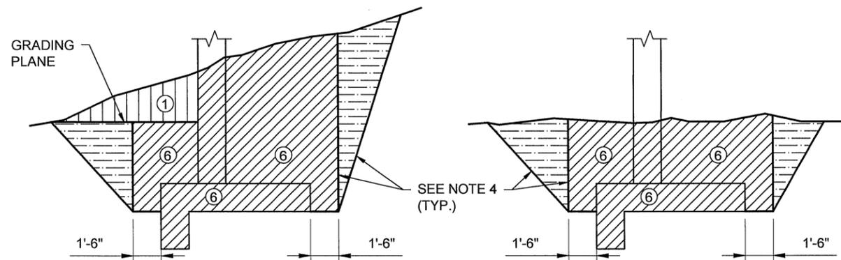
EXCAVATION FOR RETAINING WALLS
