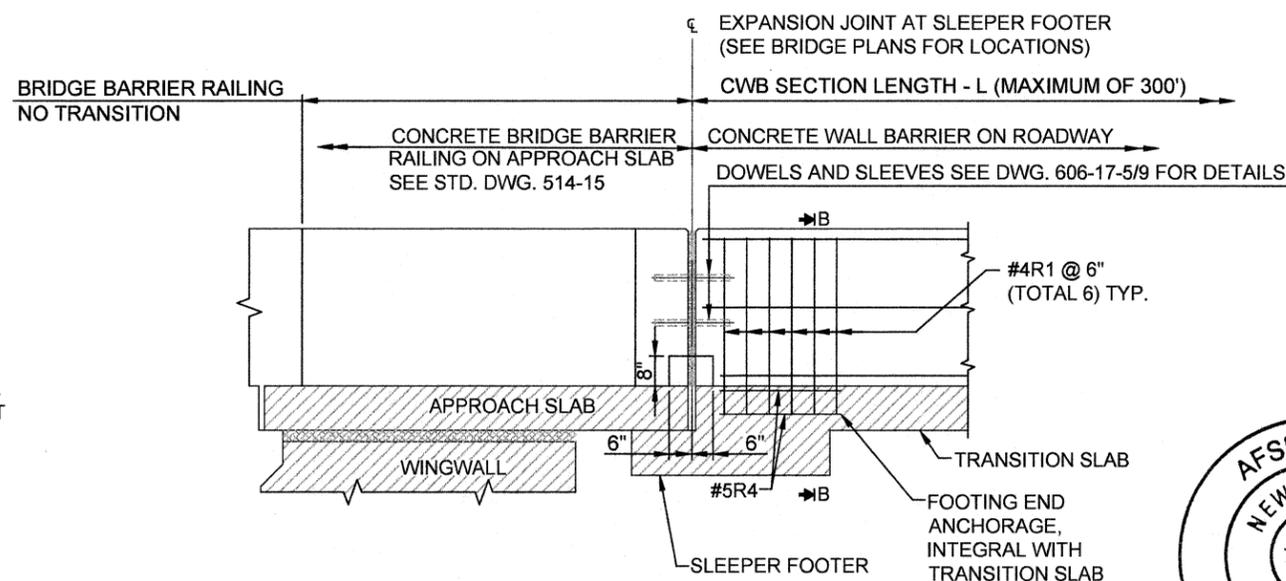
**CONNECTION OF CWB TO BRIDGE BARRIER RAILING**
