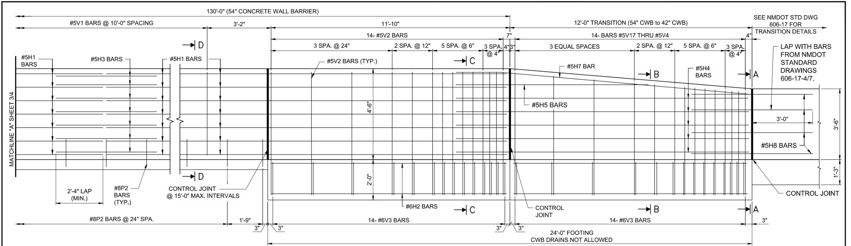
**ELEVATION - TRANSITION 54" CWB TO 42" CWB**
