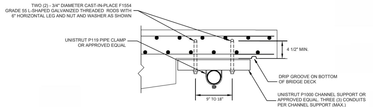
**D. TYPICAL GALVANIZED RIGID CONDUIT (GRC)
