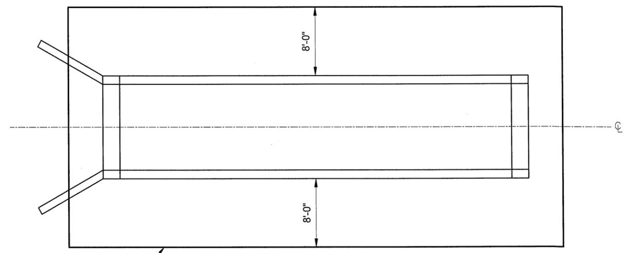
LIMITS OF MEASUREMENT FOR STRUCTURE EXCAVATION
