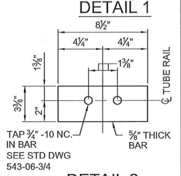
**THRIE BEAM METAL BARRIER CONNECTION TO TYPE A32 BRIDGE RAILING**
