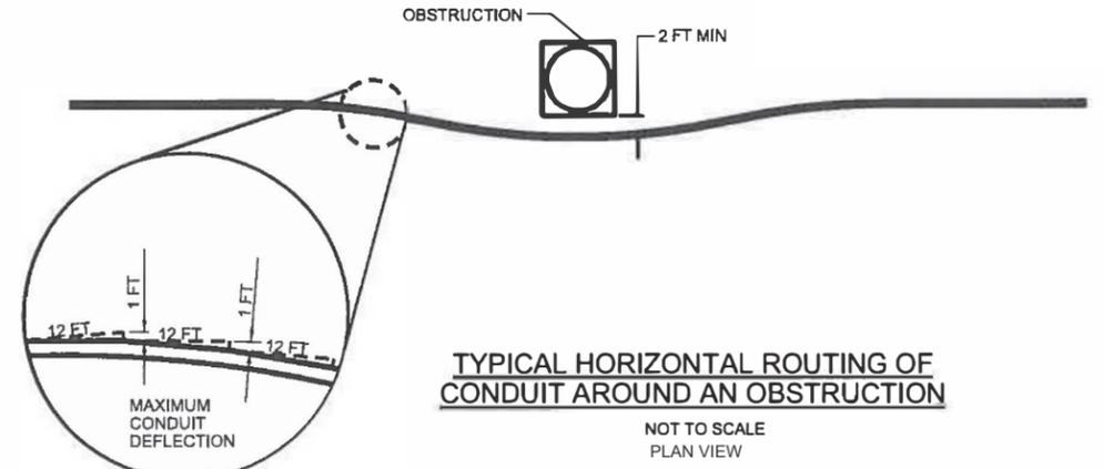
**TYPICAL HORIZONTAL ROUTING OF CONDUIT AROUND AN OBSTRUCTION**
