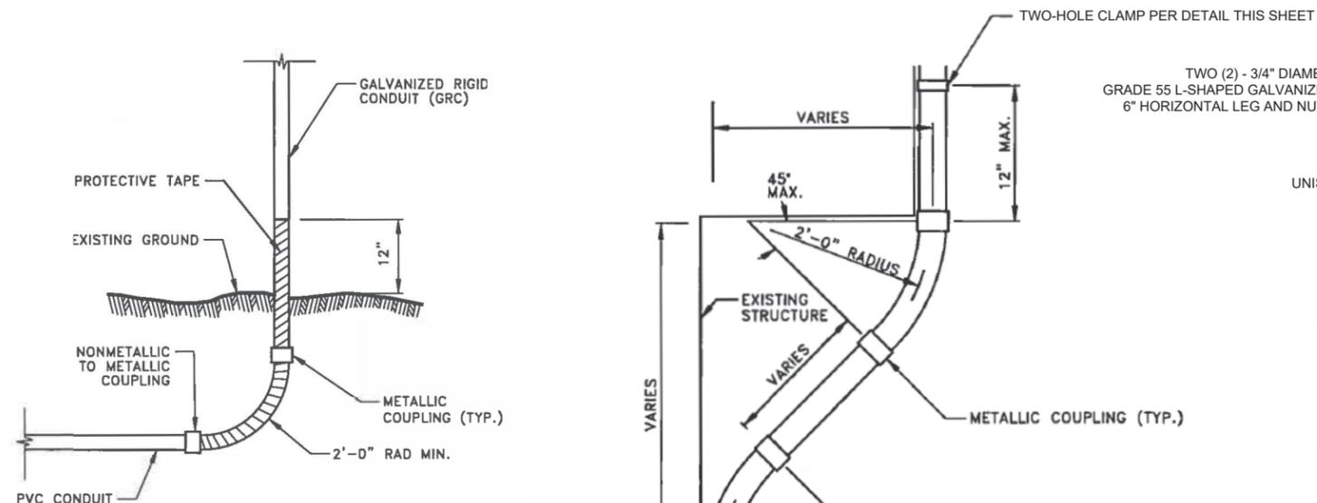
**B. TYPICAL PVC TO GALVANIZED RIGID CONDUIT (GRC)
