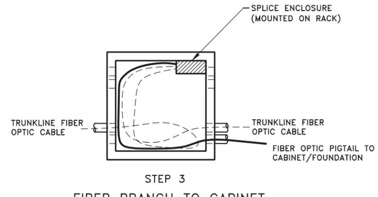
FIBER OPTIC SPLICE PROCEDURE (TOP VIEW)
