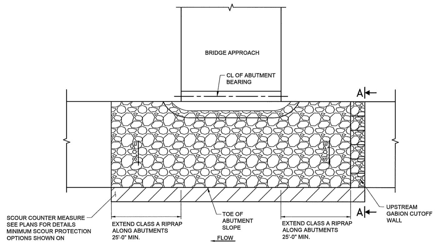
**ABUTMENTS AT EDGE OF CHANNEL**
