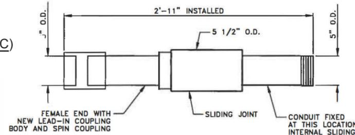
**F. TYPICAL EXPANSION JOINT PLACEMENT DETAIL**
