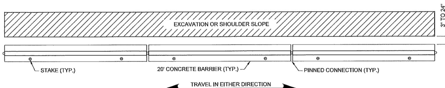
**STAKING CONFIGURATION ADJACENT TO AN EXCAVATION OR SHOULDER SLOPE**
