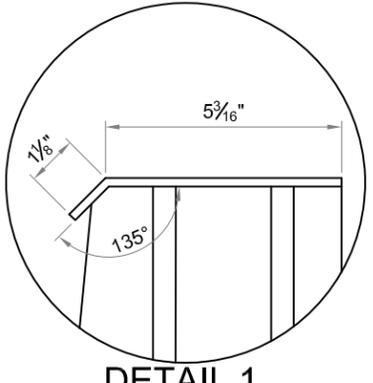
\* IT IS ACCEPTABLE TO SUBSTITUTE ANGLE IN LIEU OF BENT  $R_c$
