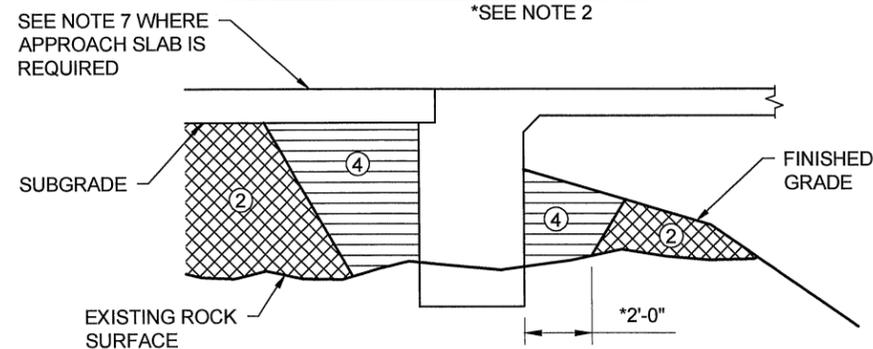
BACKFILL IN SECTION A-A: IN ROCK
