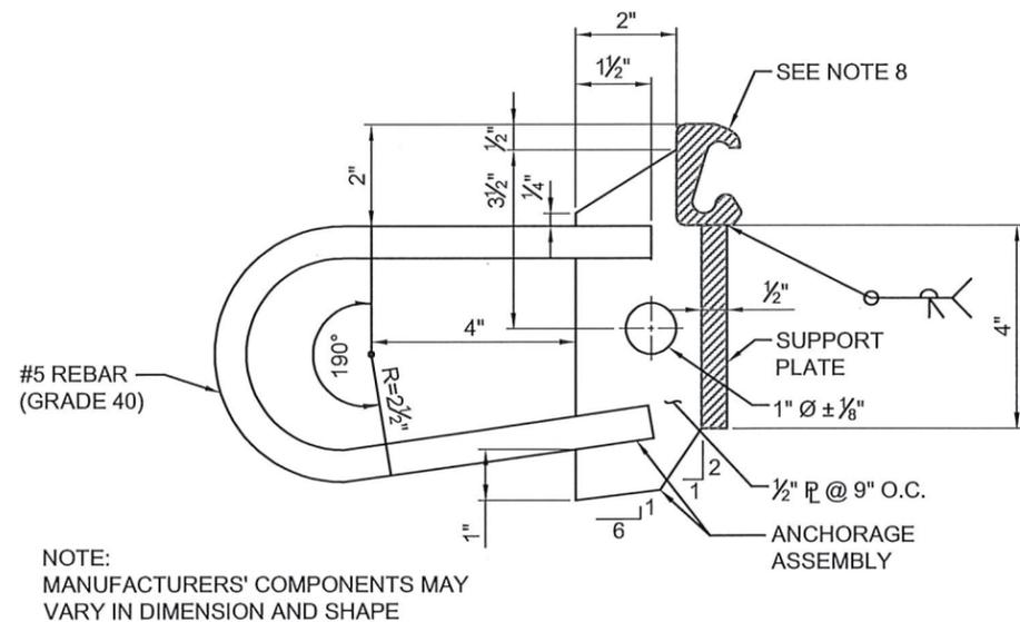
**RETAINER BAR, SUPPORT PLATE & ANCHORAGE ASSEMBLY DETAIL**
