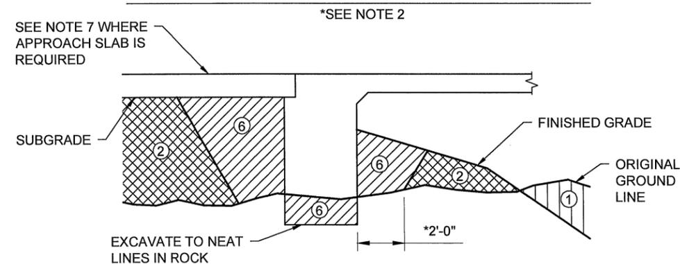
EXCAVATION IN SECTION A-A: IN ROCK
