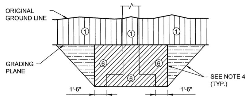
EXCAVATION IN SECTION B-B: NORMAL
