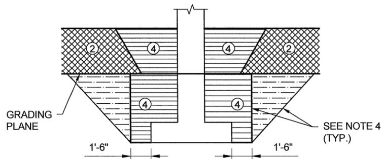
BACKFILL IN SECTION B-B: NORMAL
