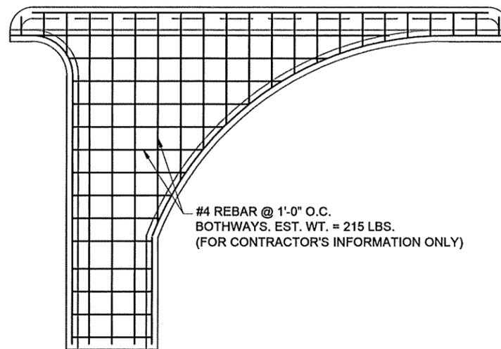
**REBAR PLACING PLAN**
