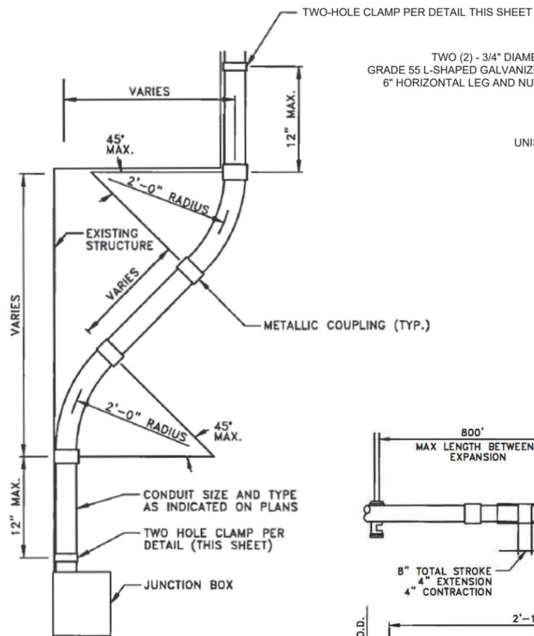
**E. TYPICAL GALVANIZED RIGID CONDUIT (GRC)
