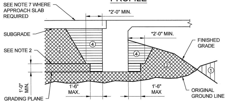
BACKFILL IN SECTION A-A: NORMAL
