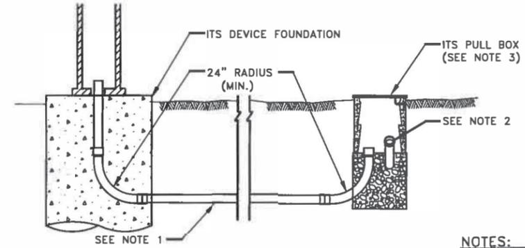
**CONDUIT ARRANGEMENT FOR ITS DEVICE FOUNDATION**
