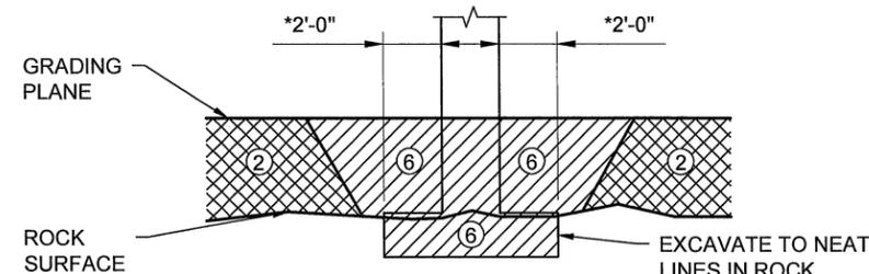
EXCAVATION IN SECTION B-B: IN ROCK
