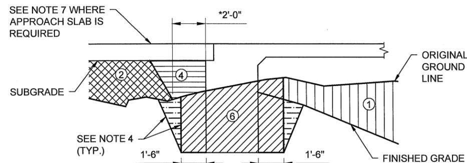
EXCAVATION IN SECTION A-A: NORMAL
