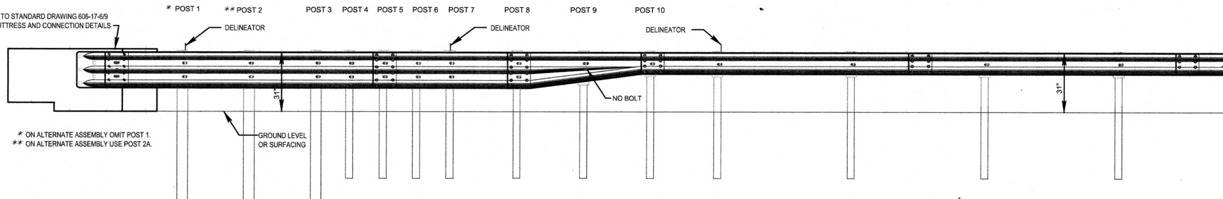
31" ELEVATION STANDARD INSTALLATION (ASYMMETRICAL SHAPE)
