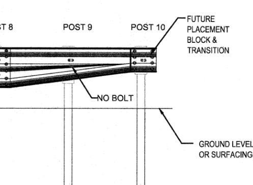
STANDARD 31" INSTALLATION USING ASYMMETRICAL SHAPE TRANSITION
