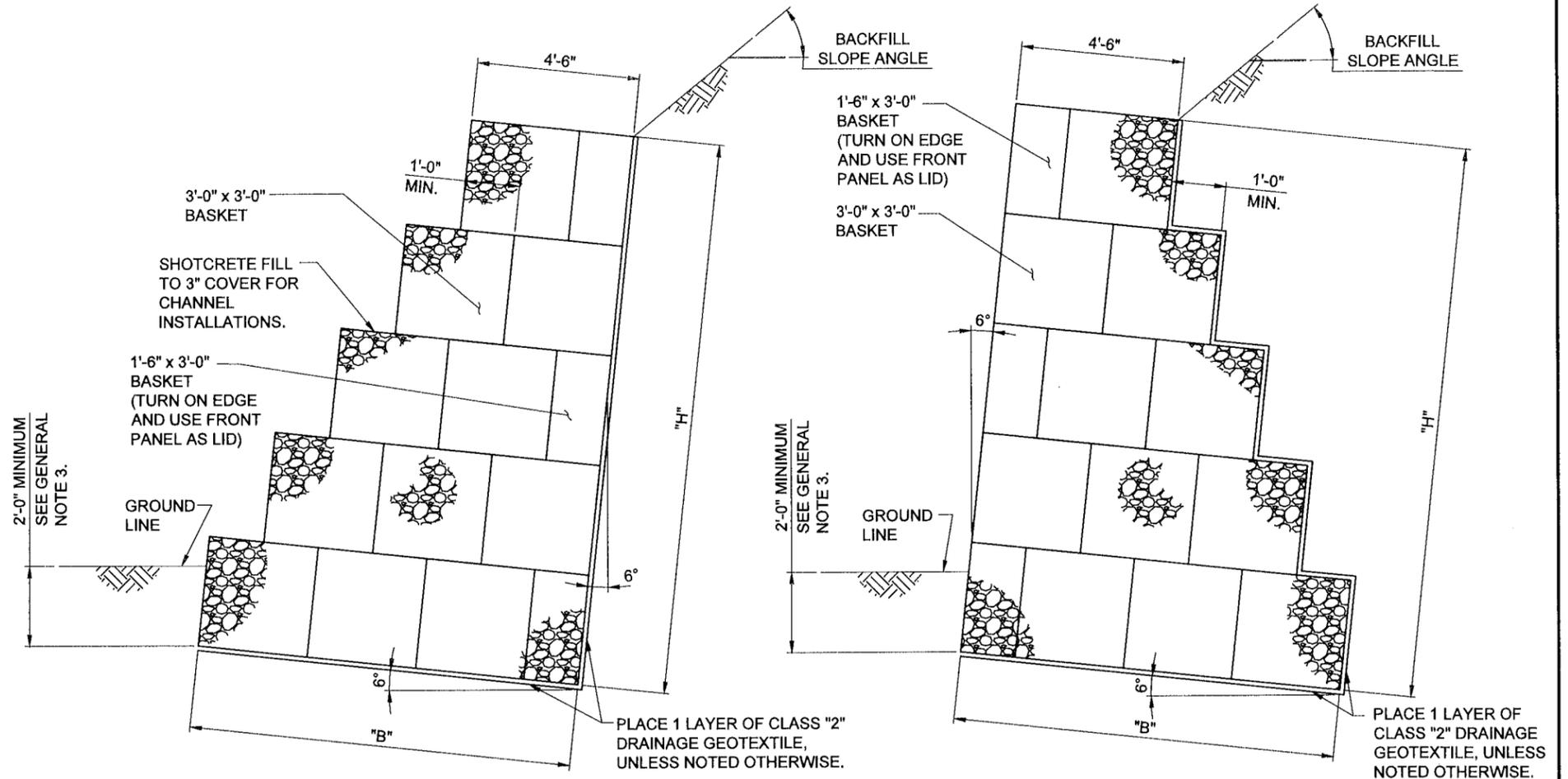
TYPICAL CROSS SECTION FOR TYPE "A" STANDARD RETAINING WALL
