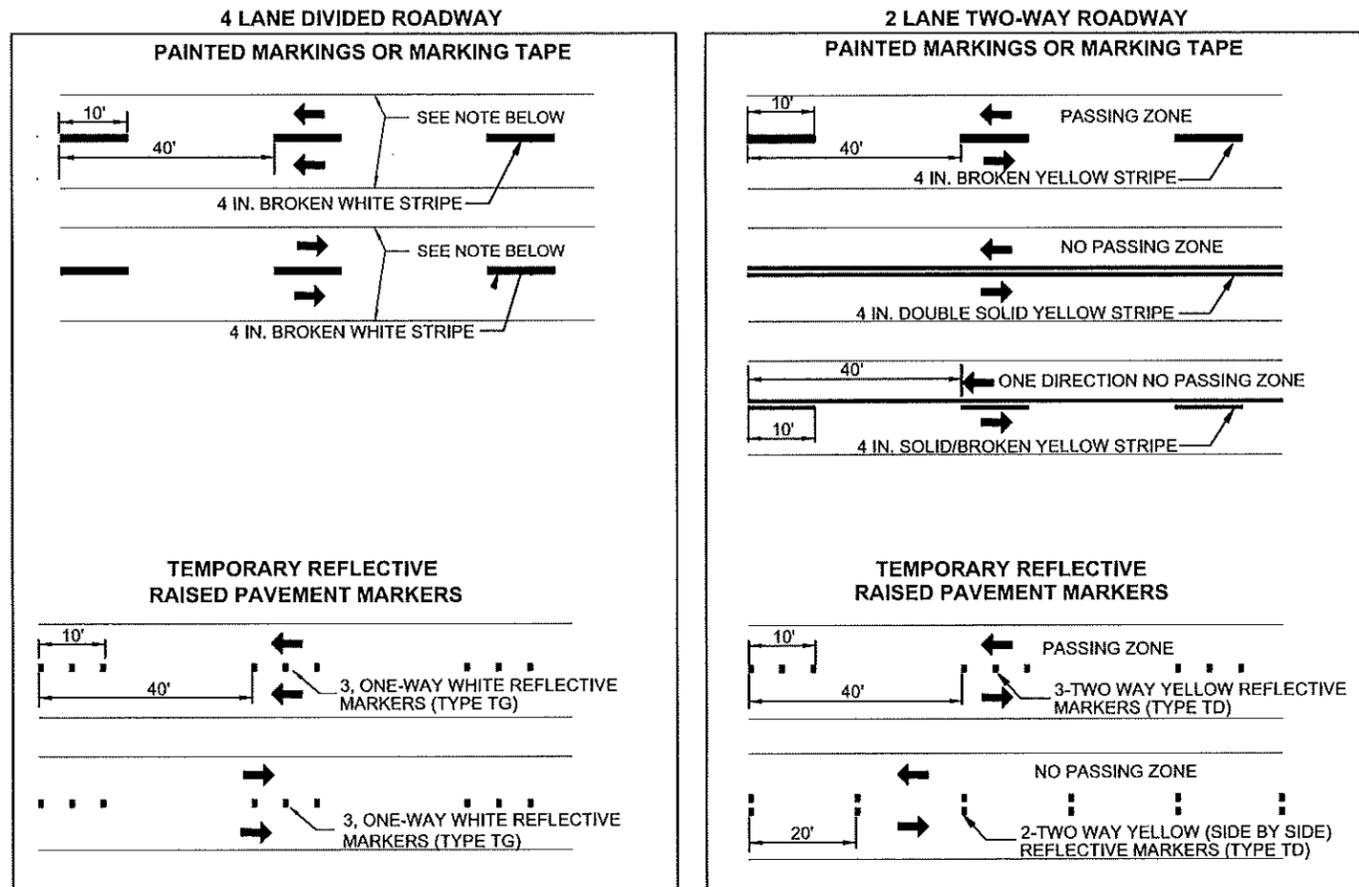
NOTE: EDGE LINES SHALL BE ADDED IF SHOWN IN THE CONSTRUCTION SIGNING AND STRIPING PLANS.
