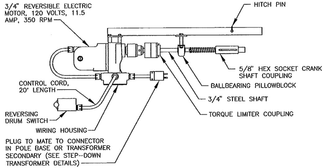
**PORTABLE DRIVE MOTOR ASSEMBLY**
